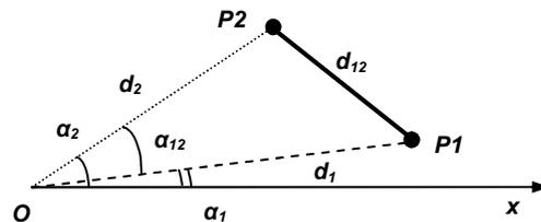
Figure 2: Diagram used for calculation of transponder speed from two consecutive measurements data.
