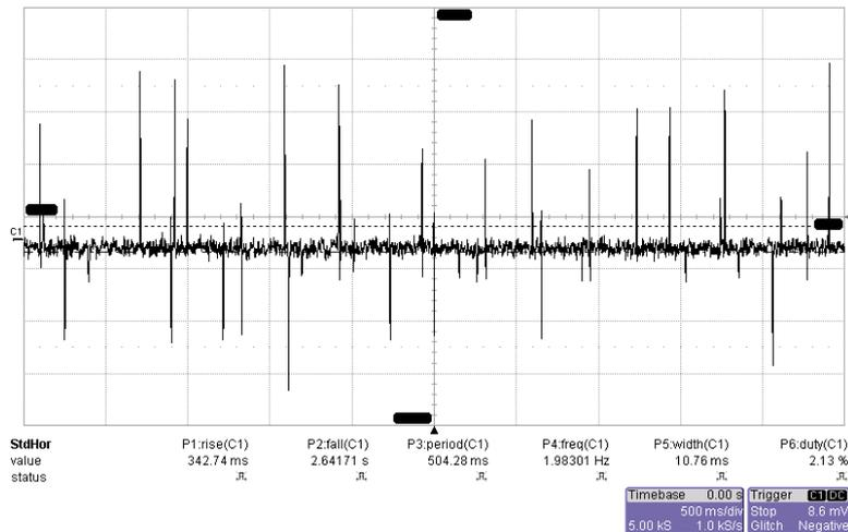
**Figure 5: The signal received by the RFID Radar when four transponder units are in the active area**
