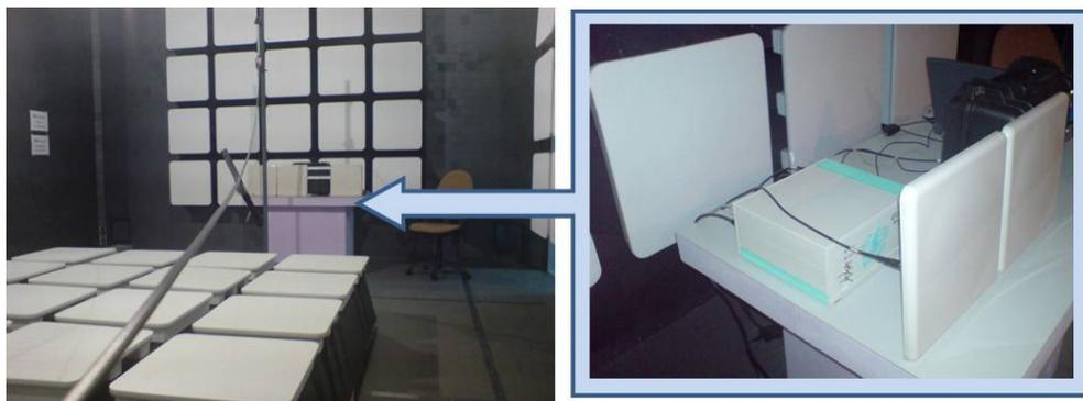
**Figure 1: Semi-anechoic chamber (left) and experimental set-up for in-door speed measurements (right).**
