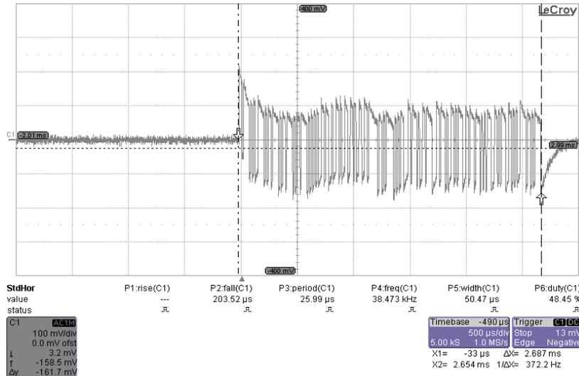
**Figure 6: The content for one transponder memory content takes 2.66 milliseconds (the demodulated signal received by the processing unit)**
