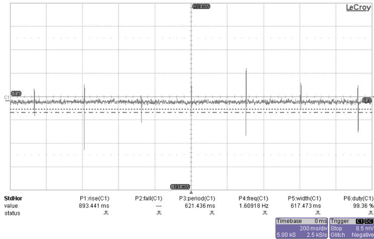
**Figure 4: The signal received by the RFID Radar when only one transponder unit is in the active area**
