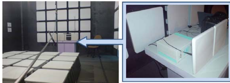
Figure 1: Semi-anechoic chamber (left) and an experimental set-up (right).
