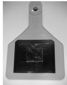
Figure 6. The label transponder attached to the animal's tag.
