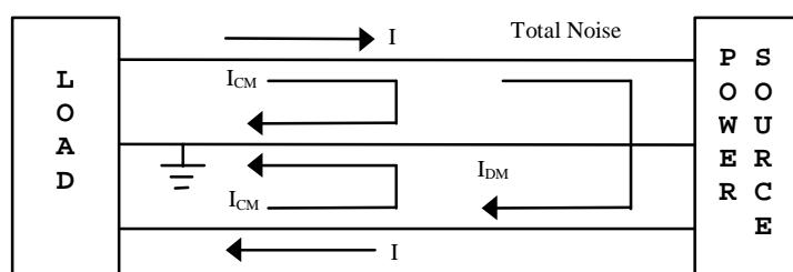
FIGURE 1. Common Mode and Differential Mode Noise Currents
