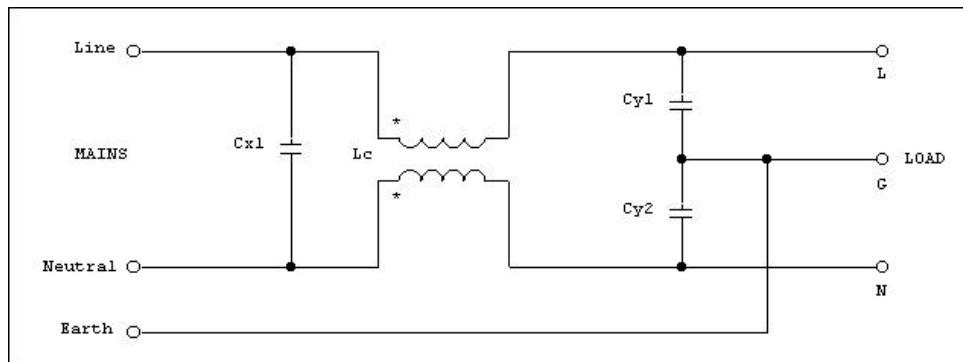
FIGURE 2. A Simple Low Cost EMI Power lines Filter
