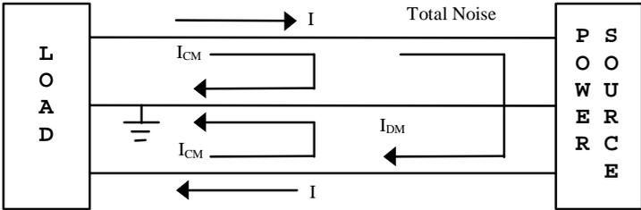
FIGURE 1. Common Mode and Differential Mode Noise Currents
