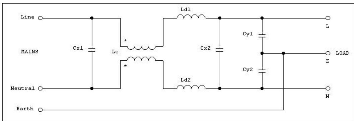
FIGURE 3. A Complete EMI Power lines Filter
