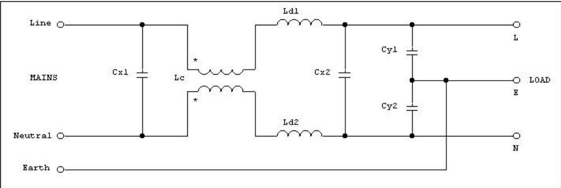
FIGURE 3. A Complete EMI Power lines Filter
