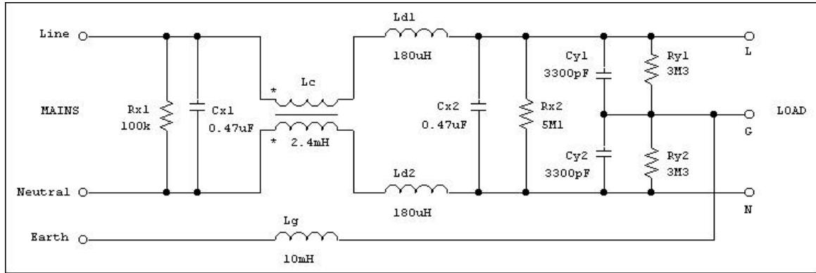
FIGURE 4. The filter used to measure the noise of a 100W forward switching power supply
