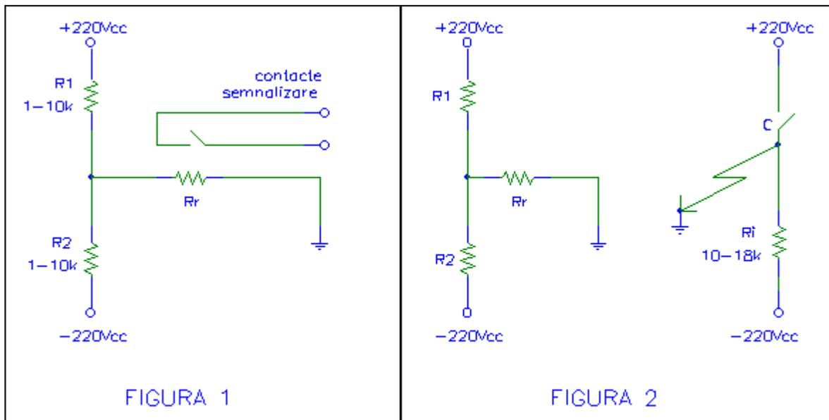
The  $R_1$  and  $R_2$  resistor have values between 1 and 10 k $\Omega$ , depending on the relay type (this is an ordinary telephone relay with an operating voltage between 24 and 48V). Figure 2 presents a circuit section where the main element is an intermediate relay  $R_i$ . This has a terminal connected to the negative voltage polarity and the other terminal is connected to the positive polarity by the mean of a relay contact C (it can be an intermediate or another type of relay).
